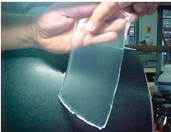
Fig. 7. Photo of (0.4/0.4/4.5) superabsorbent hydrogel composed of methacrylated cashew gum (CGMA) cut as a membrane to compressive stress measurements.
